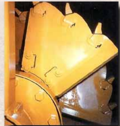
USE PADDLE AERATOR W/ OPTIONAL SPADE HI-CARBON OR CARBIDE TEETH FOR INSITU MILLING, WINDROW FORMATION & AERATION
